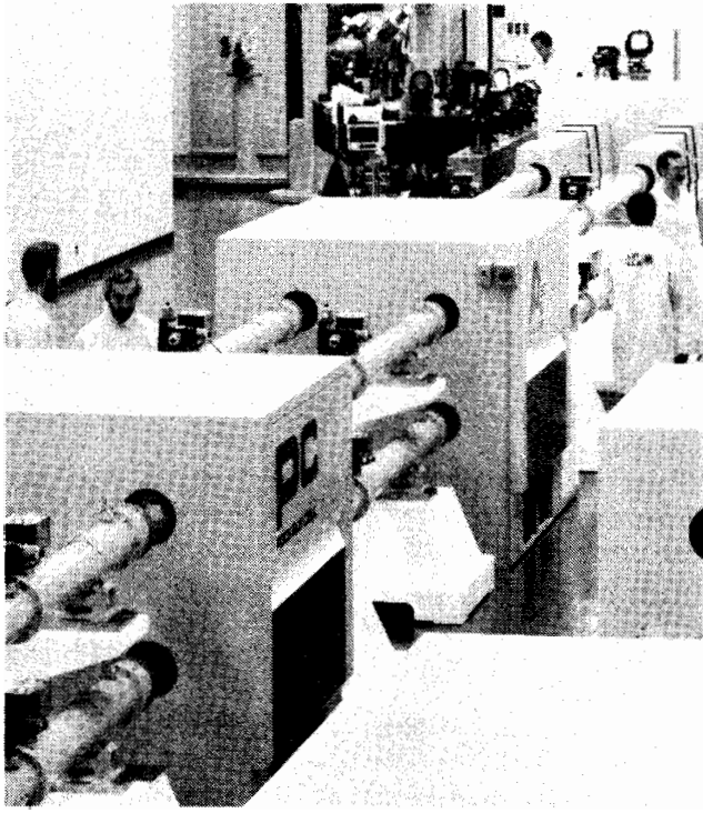
At the University of Rochester in New York State: prototype of the Omega laser now used to pump x-ray lasers.
