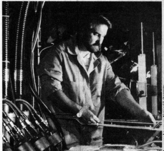
A Lawrence technician works to assemble the electron injector at the Advanced Test Accelerator (ATA), a $55 million, 50 million electron-volt, 10,000-ampere linear electron beam accelerator.
