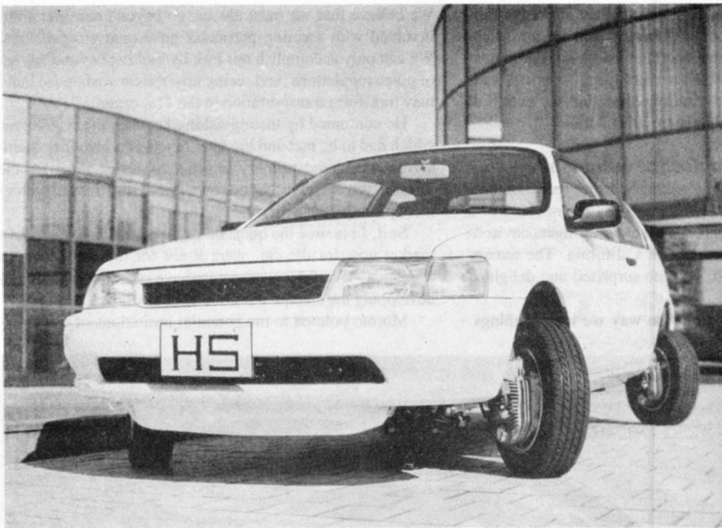
A prototype of the Japanese Equos battery-run electric car. Among other unique features, the car's wheels are independently controlled, so that they can turn in parallel to allow the driver to slide deftly into a parking place.
