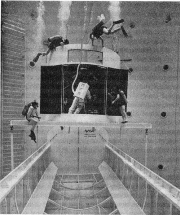
Astronauts training to effect repairs on the future Space Telescope in 1979 in the Neutral Buoyancy Simulator, a huge water tank used to simulate zero gravity, at Marshall Space Flight Center in Huntsville, Alabama. Space exploration for the new malthusians like Paul Kennedy is anathema: His ilk think it's bad enough for the Earth to be so populated with mankind, who is in the image of God; they can't bear the thought that a new Renaissance would lead people to colonize and expand on other planets as well.
