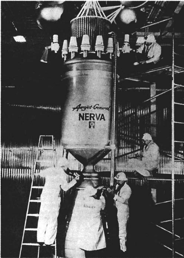
This full-scale wooden mock-up of the Nuclear Engine for Rocket Vehicle Application (NERVA) helped engineers observe the placement and orientation of components for the nuclear propulsion system. The photograph was taken in 1962. The nuclear reactors used in the NERVA program were developed at the Los Alamos National Laboratory.
