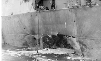
Damage sustained by the guided missile destroyer USS Cole , after a suspected terrorist bomb exploded in the port of Aden.
