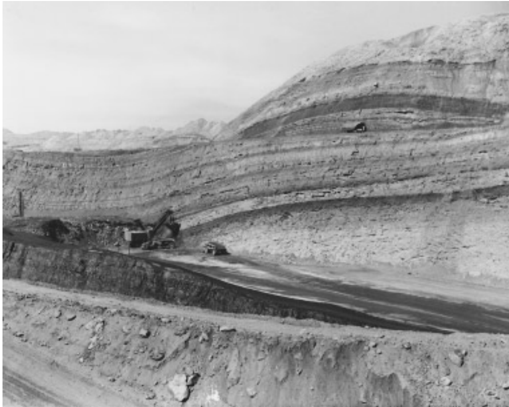
Strip-mining of coal in Wyoming. Increased use of surface-mining methods allowed the industry to proceed at a lower overall technological mode of production.
