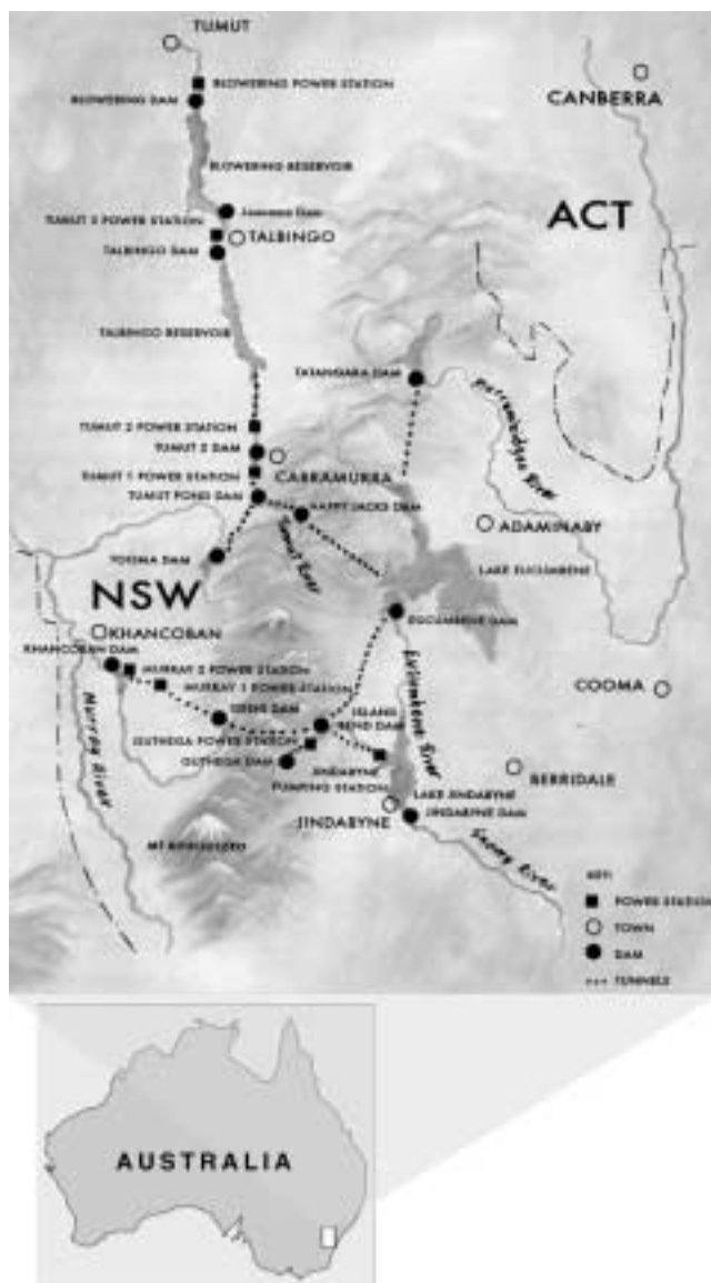
The Snowy Scheme, rated by the American Society of Engineers as "one of the seven engineering wonders" of the modern world, covers an area of 7,780 square kilometers, with 16 dams and 7 power stations.
