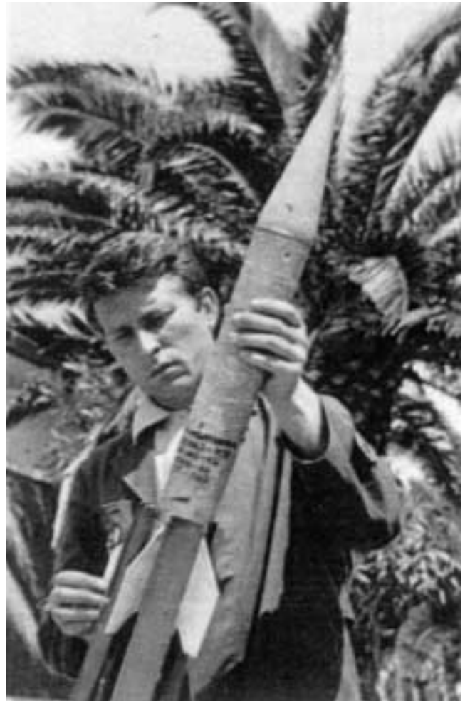
The indigenously-developed Slovenia Kamnik-1 rocket was used to seed clouds and suppress the formation of hail during thunderstorms. The program, itself, was later suppressed by the Yugoslav military.
