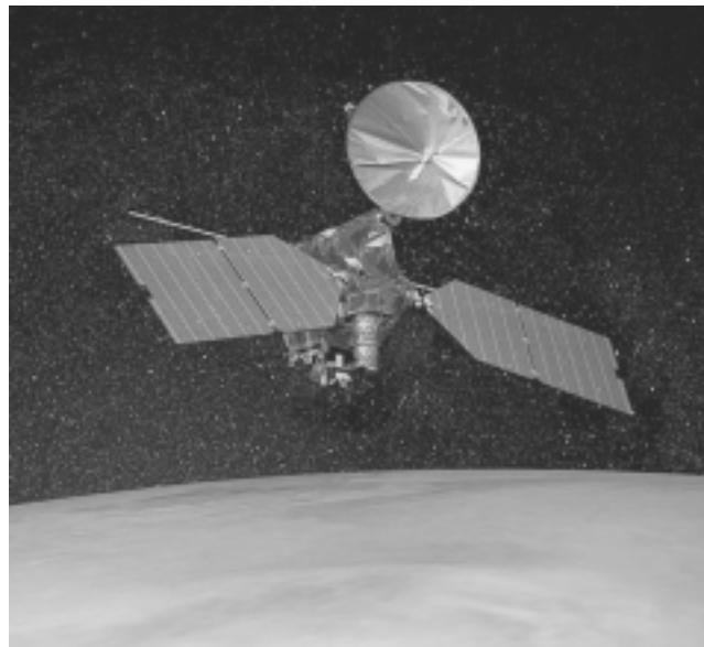
The next spacecraft bound for Mars in NASA's campaign, will be the Mars Reconnaissance Orbiter, to launch in 2005. It will be able to image the landscape to see details as small as a table, will scan for underground layers of water and ice, and will identify surface minerals. Scientists will use what they have learned from the rovers on the ground, to refine their search from orbit.
