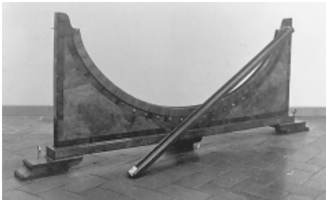
(a) A brachistochrone model built by Francesco Spighi in the 17th Century. A ball that rolls down the cycloidal track reaches the bottom faster than one rolling down the straight track.
