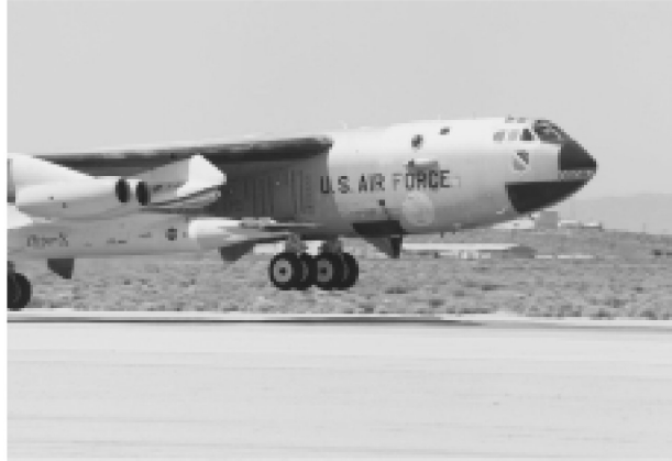
Launch aircraft takes off in March, carrying the hypersonic X-43A research plane on its wing for high-altitude launch.
