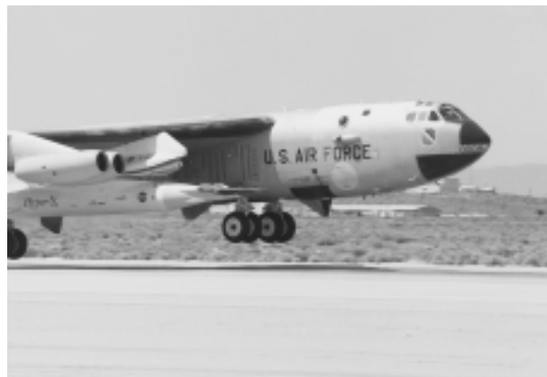
Launch aircraft takes off in March, carrying the hypersonic X-43A research plane on its wing for high-altitude launch.
