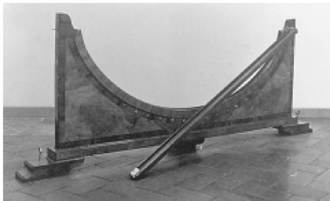
A brachistochrone model built by Francesco Spighi in the 17th Century. A ball that rolls down the cycloidal track reaches the bottom faster than one rolling down the straight track.
