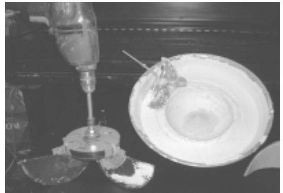
The torus-building machine tool, and its product.
