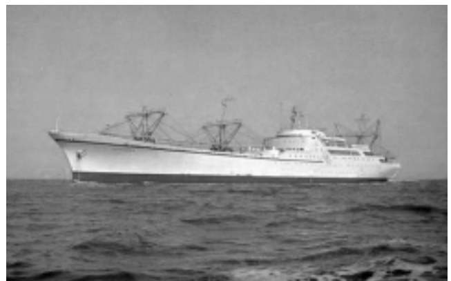
The NS Savannah was the first nuclear-powered cargo/passenger ship. She was a product of Atoms for Peace optimism, designed to demonstrate the technical feasibility of nuclear merchant ships. NS Savannah could circle the globe 14 times at 20 knots without refueling. Nuclear surface ships, submarines, and icebreakers all use nuclear desalination for their plant and potable freshwater needs.
