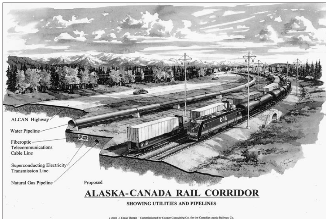
This artist's conception shows the railroad running alongside the AlCan Highway, along with utility, gas, and water lines. It was commissioned in 2002 by Cooper Consulting Co., for the Canadian Arctic Railway, which sponsored the two-year feasibility study for the Alaska-Canada Rail Corridor.
