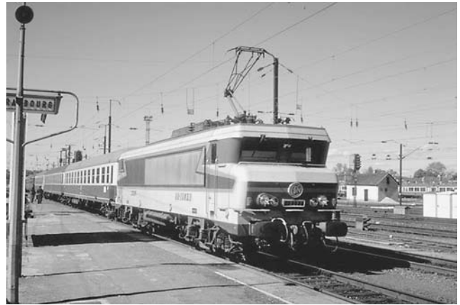
High-speed railroad travel and freight requires electric-powered locomotives, whose mounted pantograph devices pull power from overhead lines. This means construction of new power facilities, substations, and transmission lines, as well as rail, because the United States has lost virtually all the electrified rail mileage it once had.
