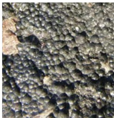
A sample of pitchblende, the ore containing uranium that Marie and Pierre Curie obtained from Bohemia. The Curies devised a way to separate out the uranium from the mass of pitchblende and were astonished to find that the remaining ore exhibited more radioactivity than did the pure uranium.
