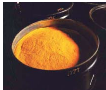
Uranium oxide (known as yellowcake), is the raw material processed into nuclear fuel. It is converted to a gas and then "enriched" through gaseous diffusion or centrifuge processing to concentrate the fissionable uranium isotope, U-235. The non-fissionable isotope, U-238, constitutes all but 0.7% of natural uranium. Reactor fuel generally requires about 3-5% of U-235.
