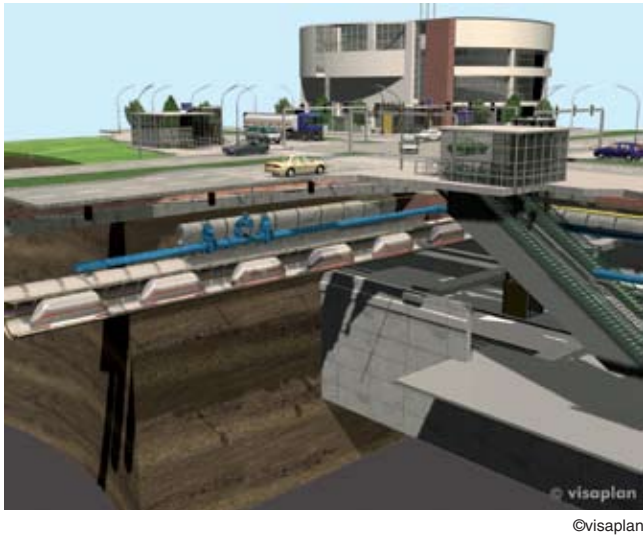
Figure 7. The Cargo Cap proposal for underground transportation of freight.
