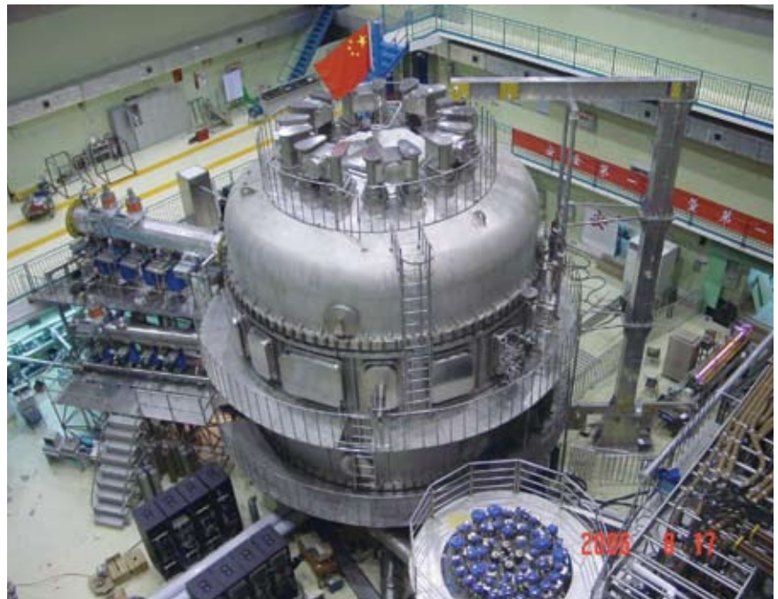
China's Experimental Advanced Superconducting Tokamak fusion device undergoes testing at the Institute of Plasma Physics in Hefei.
