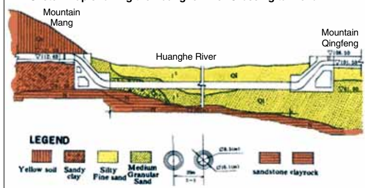
Sketch map showing the Huanghe River-Crossing tunnel of MRP
