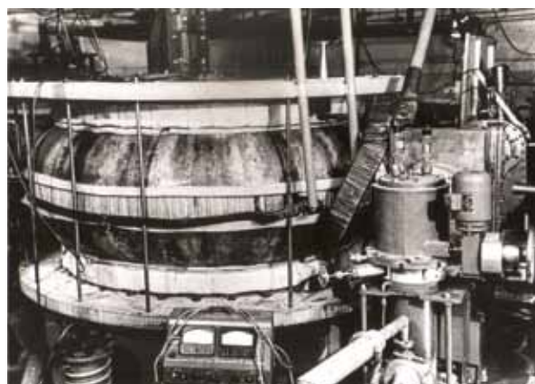
Left: Basic tokamak design. The tokamak features two external magnetic fields (toroidal and poloidal) designed to contain the plasma long enough for fusion reactions to occur. Above: The first tokamak, T-1, in the Soviet Union.
