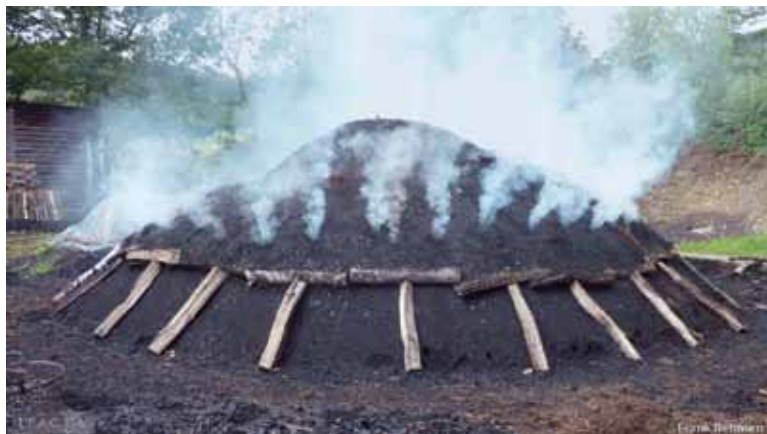
Creating charcoal by burning wood without air, under a covering of earth.
