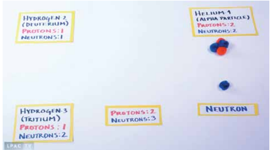
The fusion products of combining deuterium and tritium are an alpha particle (2 protons and 2 neutrons) and an extra neutron. This neutron is problematic, because it cannot be controlled by magnetic or electric fields, and collides with the walls of the fusion apparatus, creating heat and damaging the material.
