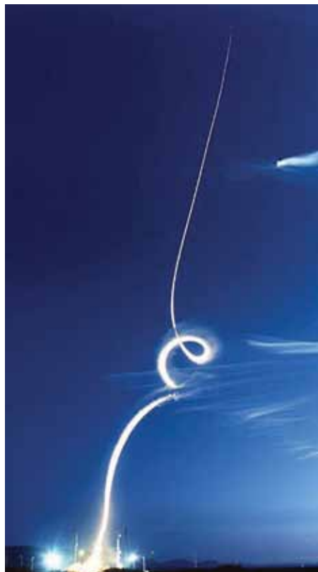
A test of the American THAAD anti-missile system at White Sands, N.M. The U.S. wanted to install these in South Korea, but Seoul has decided to build its own system instead. This corkscrew maneuver was required because the missile’s range is too large for the test site; the corkscrew trajectory prevents it from building up too much kinetic energy, and the missile falls to earth within the test area. Seoul has pointed out that such a powerful missile is not needed to defend against neighboring North Korea.
