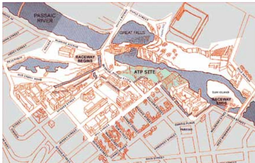
Hamilton's Vision: A schematic of Hamilton's plan for the Society for Establishing Useful Manufactures, built on the Passaic Falls (Great Falls), New Jersey. The design for the advanced waterworks and manufacturing complex was done by Pierre L'Enfant. The ATP site stands for Allied Textile Printing, and is the location of the SEUM's original textile mills, which were in operation for 200 years.
