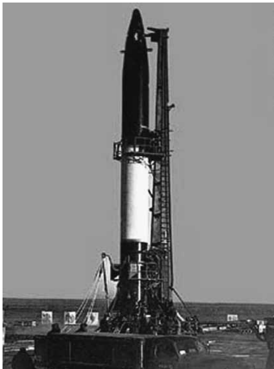
The Dong Feng-1, developed under Qian's guidance, seen here, was based on the Soviet R2 missile, itself a derivative of the German V-2 rocket.
