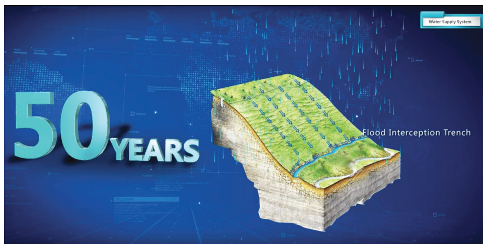
Flood interception trenches handle water levels happening rarely in 50 years.
