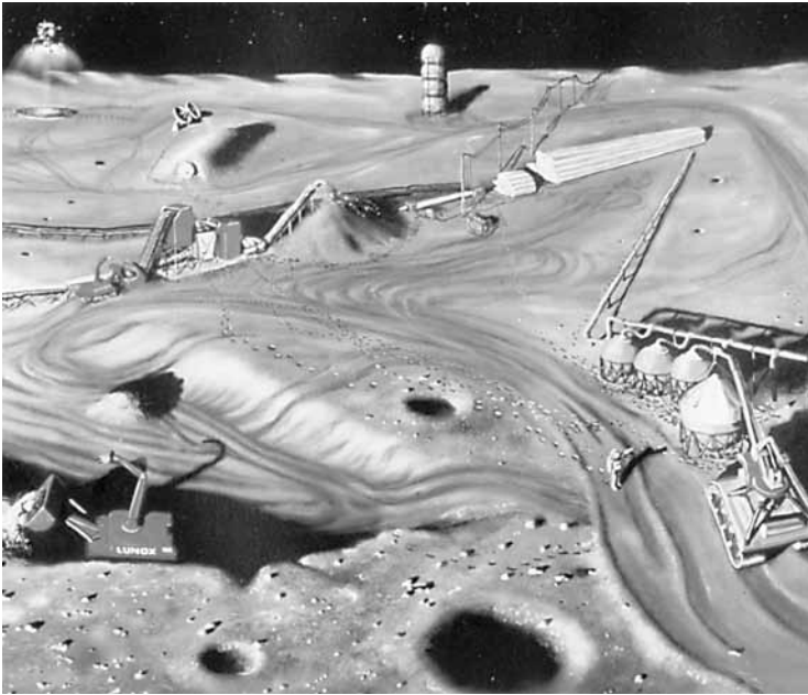
The process of lunar industrialization prepared the way for colonizing Mars. Here, a lunar resource processing pilot plant, designed to develop the technologies used for collection, analysis, and both mechanical and electrochemical separation of lunar surface resources; for production of materials needed for life support and propulsion (such as oxygen); and fabrication and construction of structural elements.
