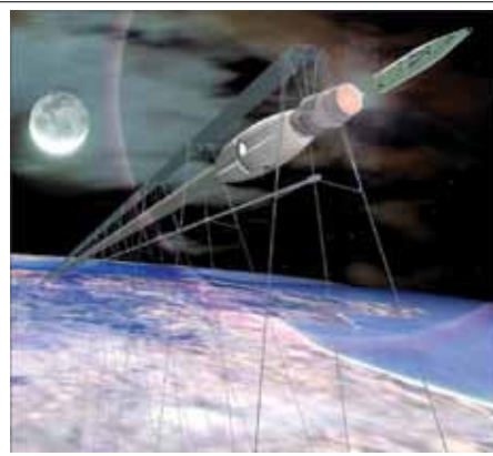
Illustration of space-launch device using maglev propulsion in a vacuum tube.
