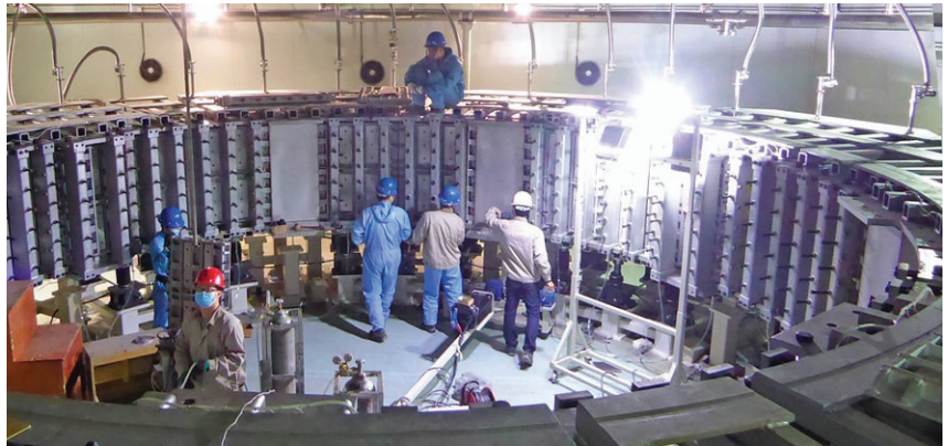
Technicians in Hefei, China, nearing completion of the poloidal field coils for insertion into the International Thermonuclear Experimental Reactor (ITER) in France.
