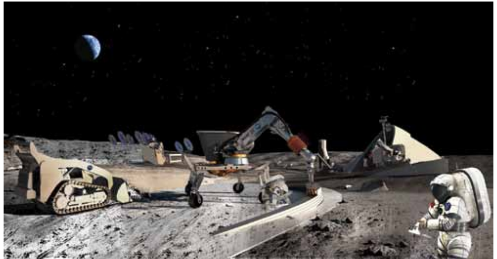
Artist’s concept for a lunar base built through in-situ resource utilization (ISRU) and a form of 3D printing known as contour-crafting.
