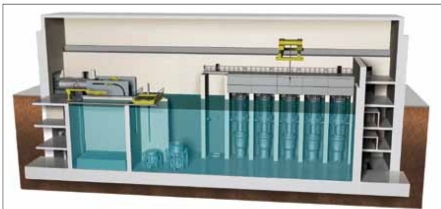
Artist’s rendering of a cross-section of a NuScale SMR power plant, showing five reactor modules installed in a below-grade pool of cooling water: NuScale’s 60 MW reactor modules are designed to be installed individually or in arrays of up to 12 units in a single plant.
