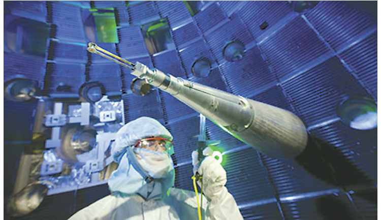
A technician works on a target positioner inside the National Ignition Facility (NIF) target chamber.
