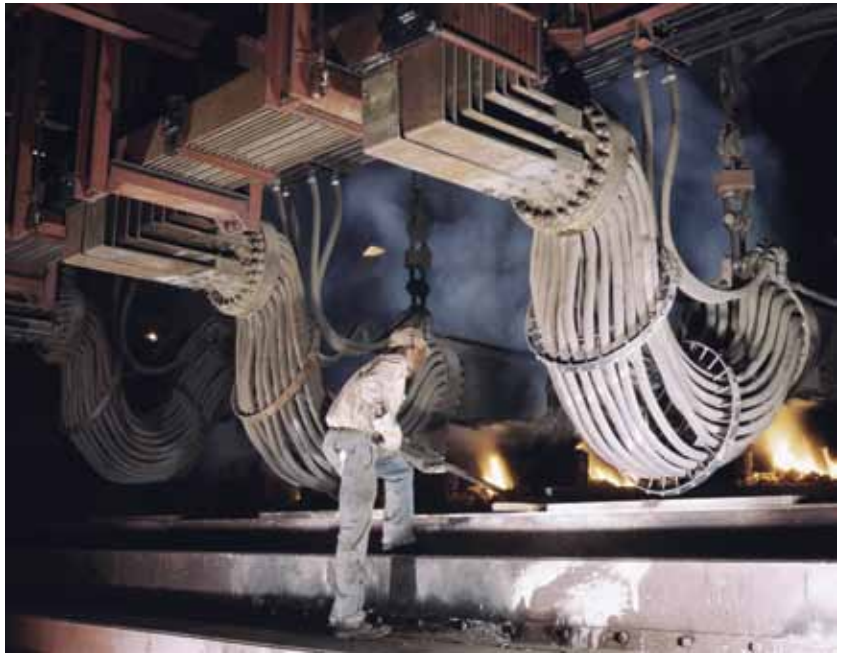
A large electric phosphate smelting furnace used in the making of elemental phosphorus, in a TVA chemical plant in the Muscle Shoals area, Alabama, June 1942.
