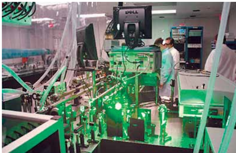
The Texas Petawatt Laser seen here was completed with the help of teams from Lawrence Livermore National Laboratory. It is a 150 joule, 140 femtosecond laser. Currently, the laser allows scientists to study states of matter such as high energy-density plasma states, similar to those found in our Sun and in supernovae.
