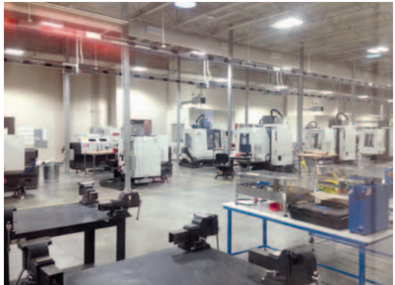
A community college manufacturing lab in Houston, Texas, showing machine tools driven by computer numerical control (CNC).
