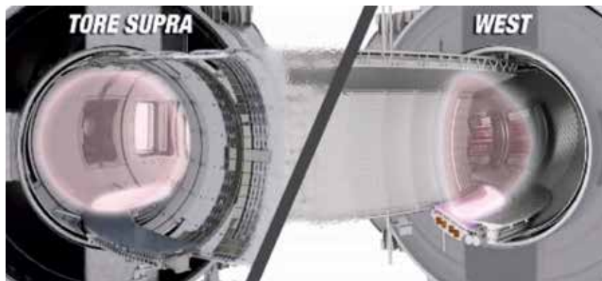
This diagram from the French Institute for the Study of Magnetic Fusion Research shows the transition in the magnetically bounded shape of an energetic plasma, from a circular cross-section in the Tore SUPRA to a D-shaped one in the WEST tokamak.
