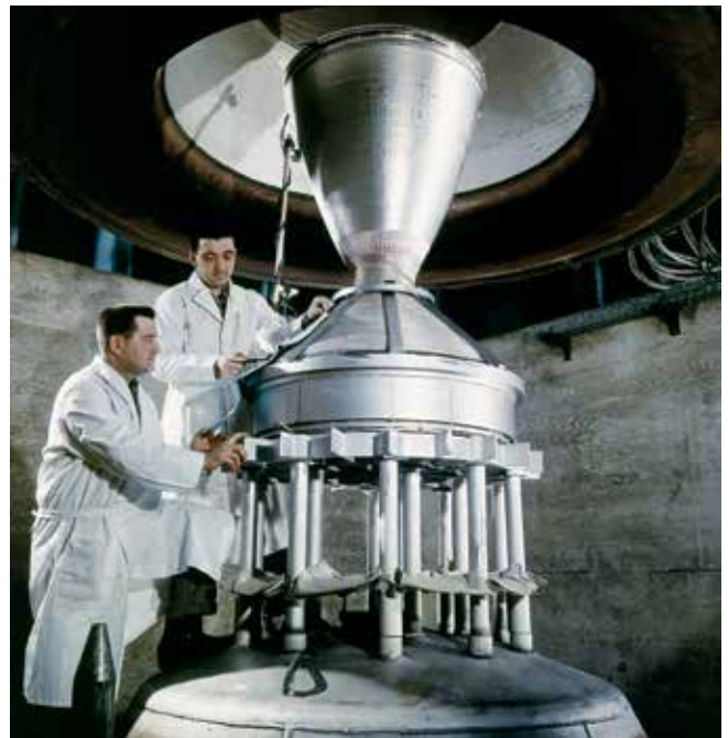
As part of NERVA, the U.S. project for a Nuclear Engine for Rocket Vehicle Applications, technicians at NASA's Lewis Research Center prepare a rocket nozzle for testing in 1964. The program was cancelled in 1973 after the Nixon administration savagely cut NASA's budget.
