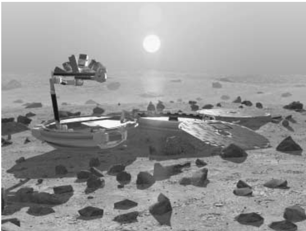
The Beagle 2 lander, carried on the European Mars Express spacecraft, will deploy a set of tiny instruments to investigate the possibility of life on Mars. At the end of its robot arm is the PAW, a collection of tools that can be rotated in to different positions, and applied to study Martian rocks and soil.
