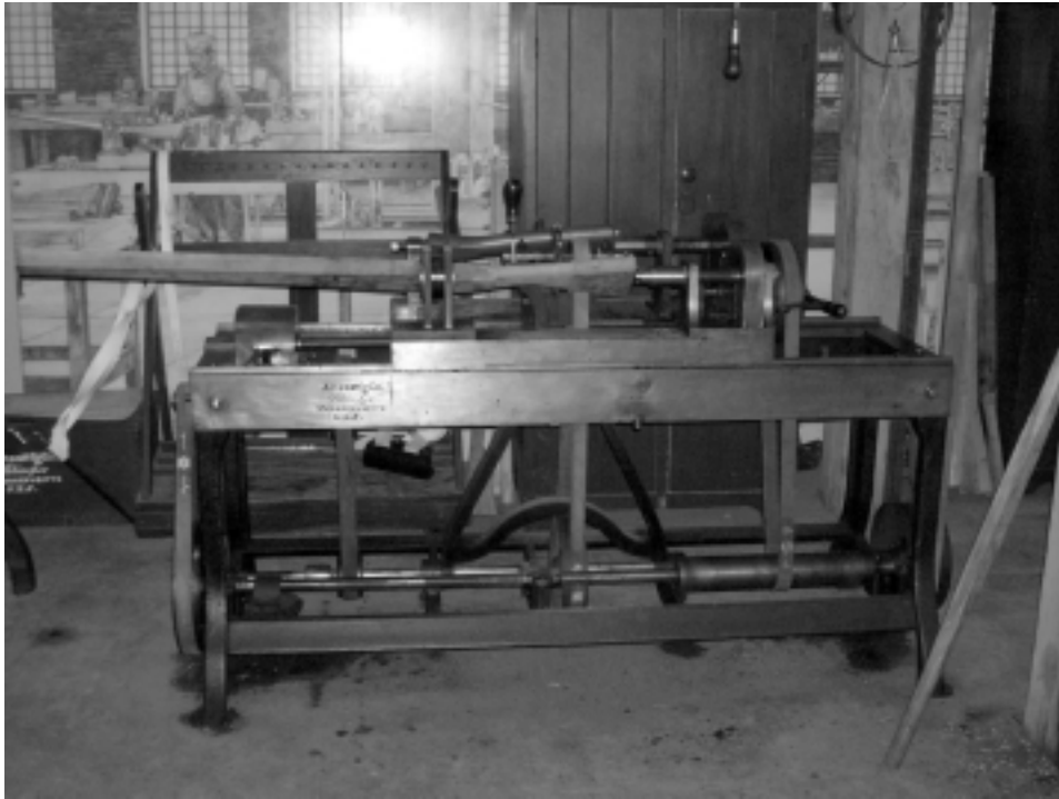
These are machine tools—lathes for gun-making—at the Harpers Ferry, West Virginia, museum. The Harpers Ferry Arsenal was established by President George Washington. It became a laboratory for checking the worth of proposed inventions.
