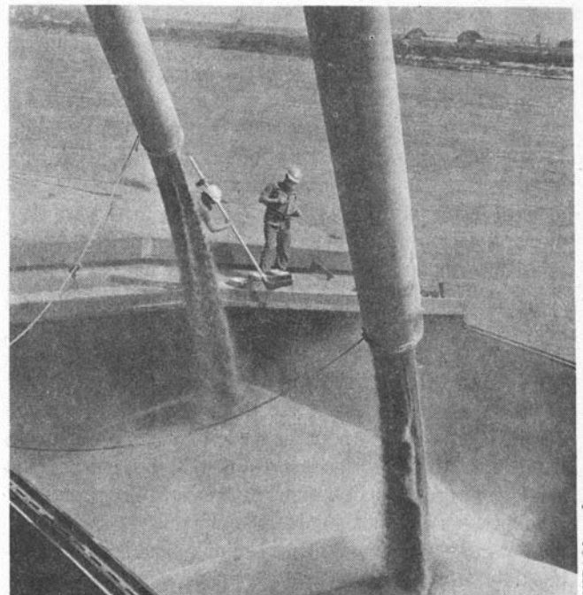
Sucker discharge grain equipment can be fitted on De Long floating piers for rapid bulk grain handling. Here grain is loaded onto barges in Kansas City.
