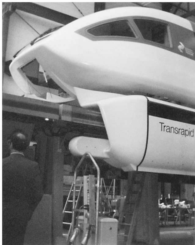
The German Transrapid, a magnetically levitated (maglev) rail system that will allow overland travel at speeds of 300 kilometers per hour or higher.
