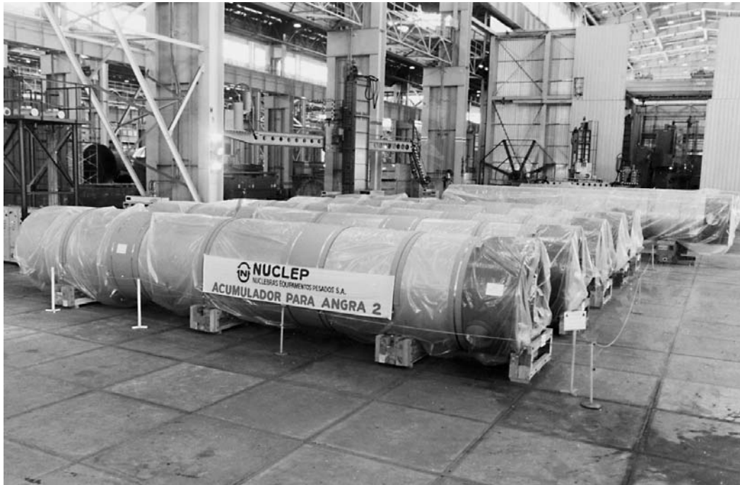
Brazil's electrical industries are among the most skilled and experienced in the world: producing the turbines for China's huge Three Gorges project, for example; and here, steam vessels for Brazil's nuclear plants at the Angra site.
