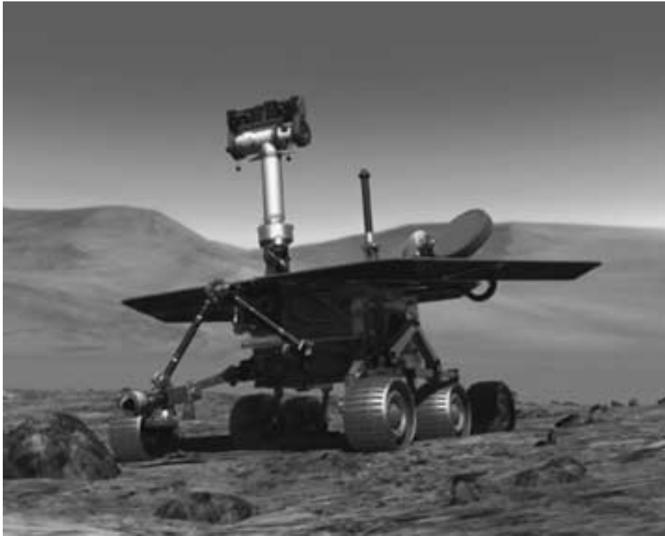
This artist's rendering of the Spirit rover on Mars shows the five-foot-tall vehicle ready to explore the red planet. Atop the mast are the two color panoramic cameras, and two black and white navigational cameras. The arm, protruding in front, houses the scientific instruments that will reveal the geologic history of Mars, by investigating the chemical, mineral, and elemental composition of Mars' soil and rocks.
