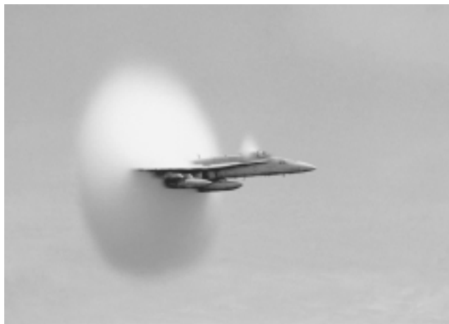
Tennenbaum showed a film of the momentary generation of a shock-wave "cloud" around the aircraft, as it breaks the sound barrier. This photograph of a U.S. Navy F/A-18 Hornet shows a moment in the process.
