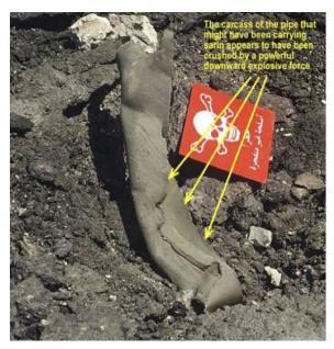
Deformation of sarin containing pipe and crater from the action of the explosive charge placed on top of the pipe.
