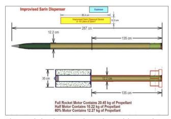
The ground-placed improvised sarin dispersal device is shown next to a standard 122 mm artillery rocket. The explosive placed on top of the pipe would cause it to be suddenly crushed, like a tube of toothpaste hit by a mallet. The sarin would be sprayed out from the metal tube.
