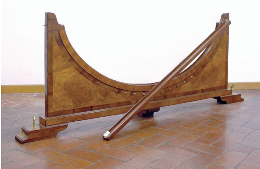
Least action pathways are not always straight lines. A brachistochrone and a pencil in water, illustrate the least action curve of a ball rolling down a track, and the least action refractive angle for light going from air to water.
