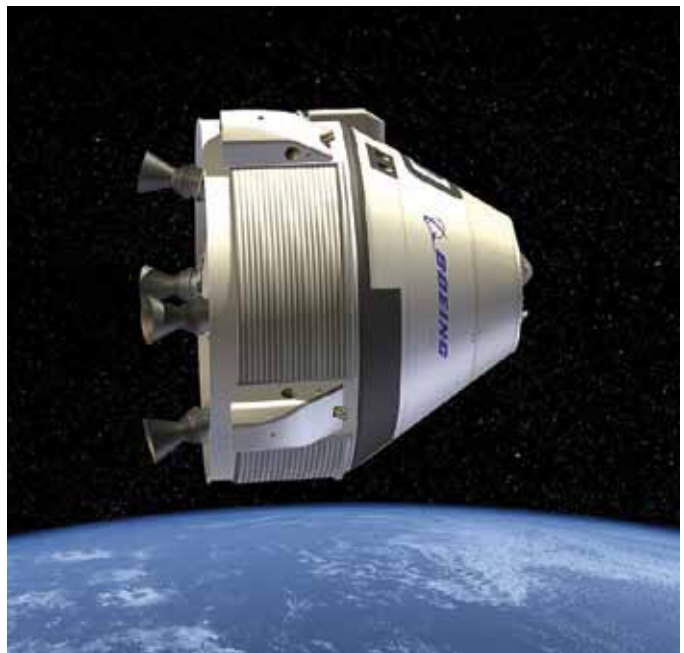
An artist’s rendering of the CST-100 Starliner showing the pusher rocket engines attached to the service module.
