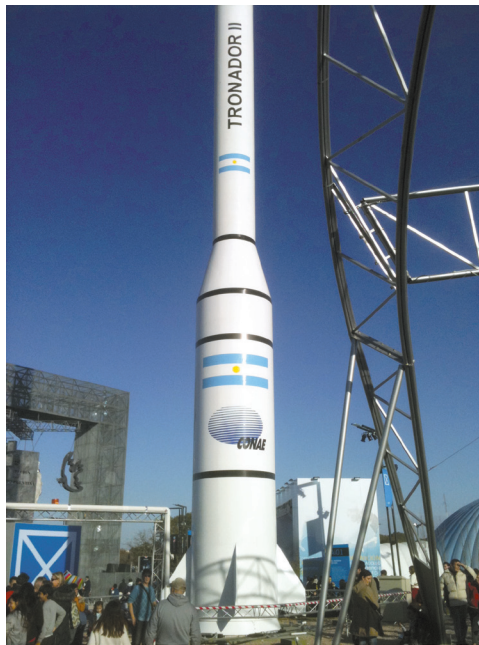
A mockup of Argentina's Tronador (Thunderer) II, a liquid-fueled rocket designed to lift payloads into Low Earth Orbit.
